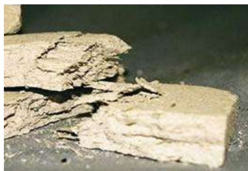
Pieces of Asbestos Insulating Board (AIB)
