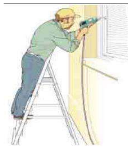
Correct – steps facing work activity
