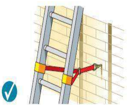
Tying near the base
